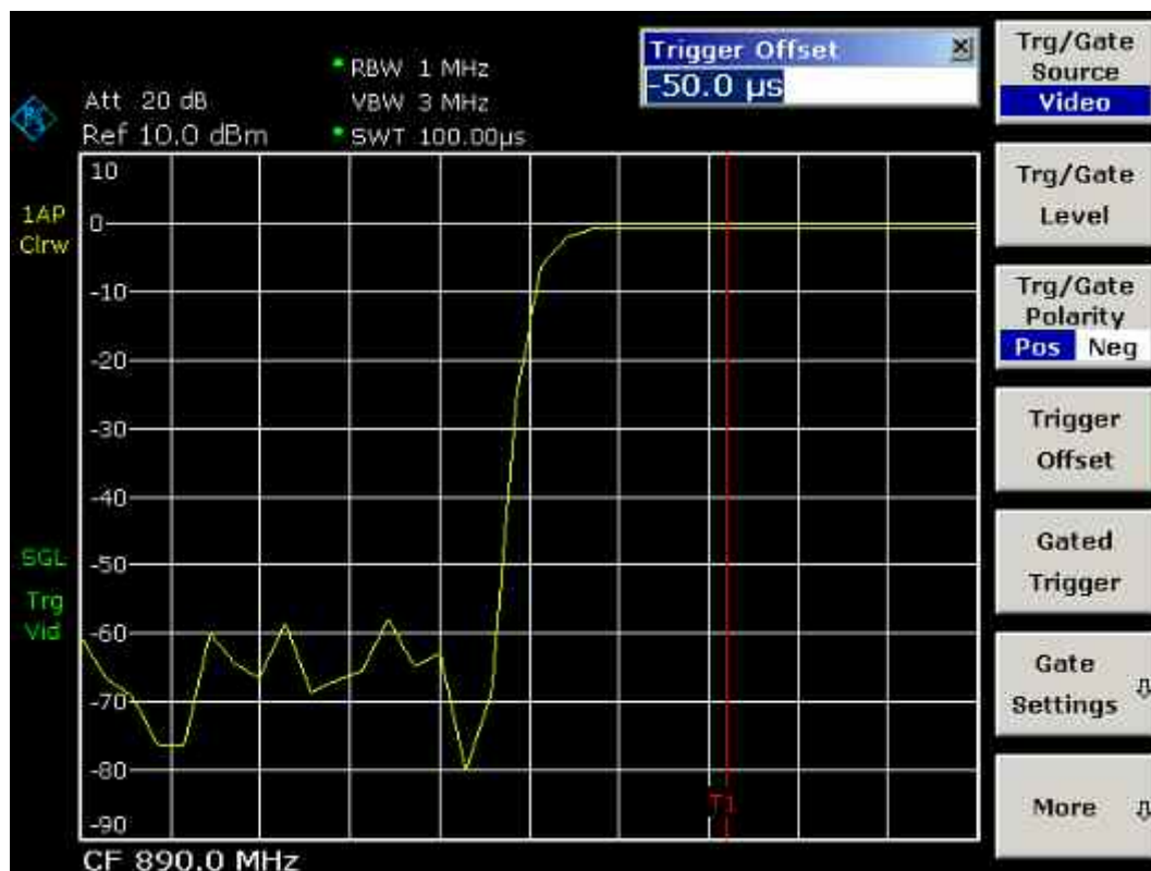
Fig. 5–10 Rising edge of the GSM burst displayed with high time resolution
